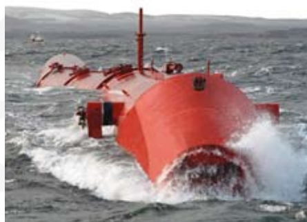
Pelamis Wave Energy Converter. Photo Pelamis Wave Power
