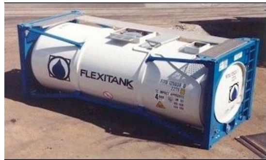
Fig 3 – Two examples of Standard Demountable Units (SDUs) built within ISO frames and easily transferable onto flatbed lorries
