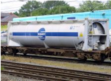
Fig 3 – Two examples of Standard Demountable Units (SDUs) built within ISO frames and easily transferable onto flatbed lorries
